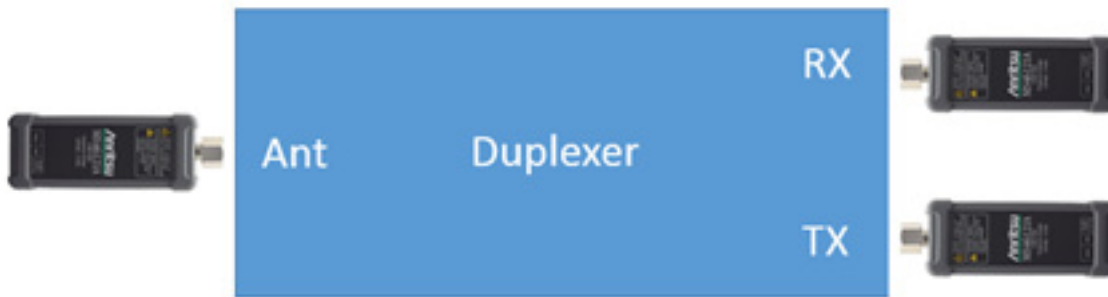
Figure 5-8. MS46121A/Bs Setup Up to Measure a 3 Port Device
